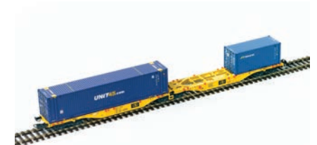
Ref. 100372 CLIP INTERMODAL Sggmrss 33 51 4961 113-9 HONEYTAK 20' DV HNKU1002713 + UNIT45 45' HC RCDU2500760
