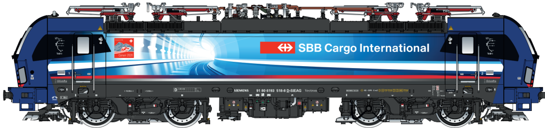
-SBB Cargo International Vectron MS, 91 80 6193 518-8 D-SIEAG, „Ticino“, 4 pantographs, equipped for D/A/CH//NL, ultramarine blue, Ceneri 2020 design, Ep.VI (2019)
