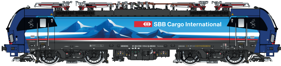
-SBB Cargo International Vectron MS, 91 80 6193 516-2 D-SIEAG, „Aare“, 4 pantographs, equipped for D/A/CH//NL, ultramarine blue, mountain design, eraVI (2019)
