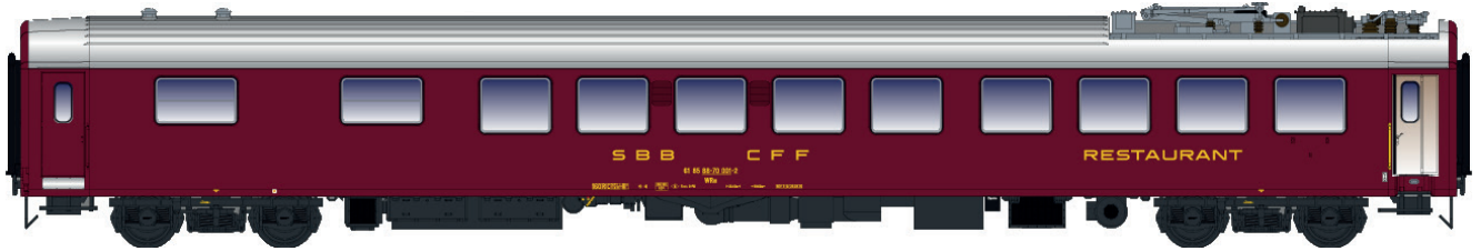
472 005 UIC-X WRm red, SBB signet, service door with window Ep.IVa
