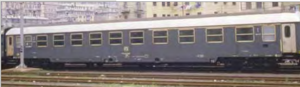
Carrozza Tipo X mista a cuccette, livrea grigio ardesia, carrelli MD. Type X first and second class couchette coach for international trains, slate gray livery, MD bogies. Typ X 1. / 2. Klasse Liegewagen für internationale Züge, schiefergraue Lackierung, MD Drehgestelle.
